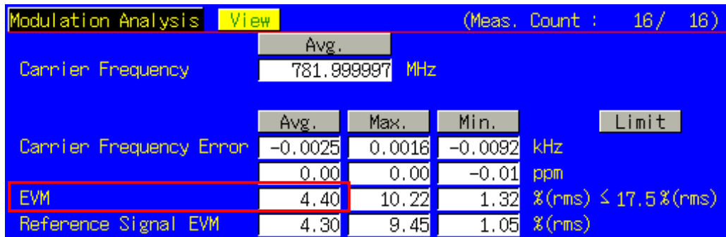
Figure 3.1.25-1 Example of Measurement Result when Test Parameter is TX3 - EVM with Exclusion Period (QPSK) (MT8820C)
